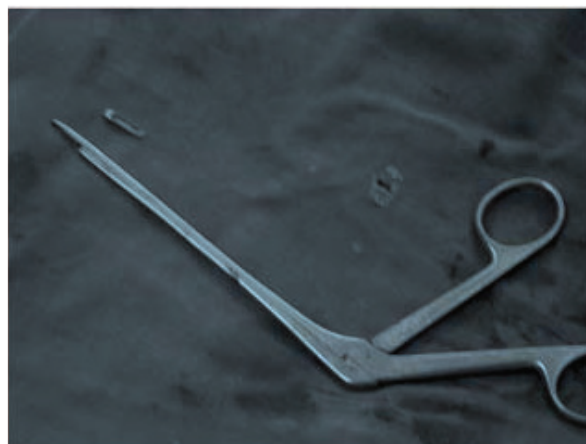
Figure 7. Photograph showing the disc forceps with broken blade.
