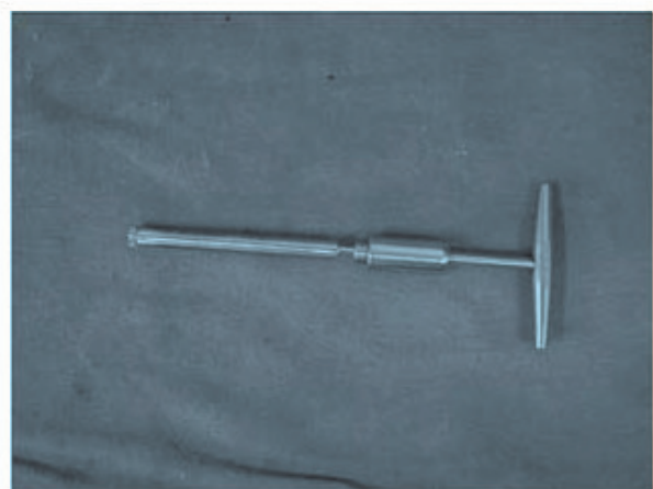
Figure 2. The broken screw removal device used to retrieve the broken metal piece.
